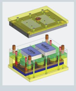
geometry for the core and cavity, which can be machined directly into the plates or separate core and cavity blocks. The core and cavity blocks are automatically sized based upon the physical part size. Solid Edge Mold Tooling can also import predefined parting surfaces in a partial or completed state.
